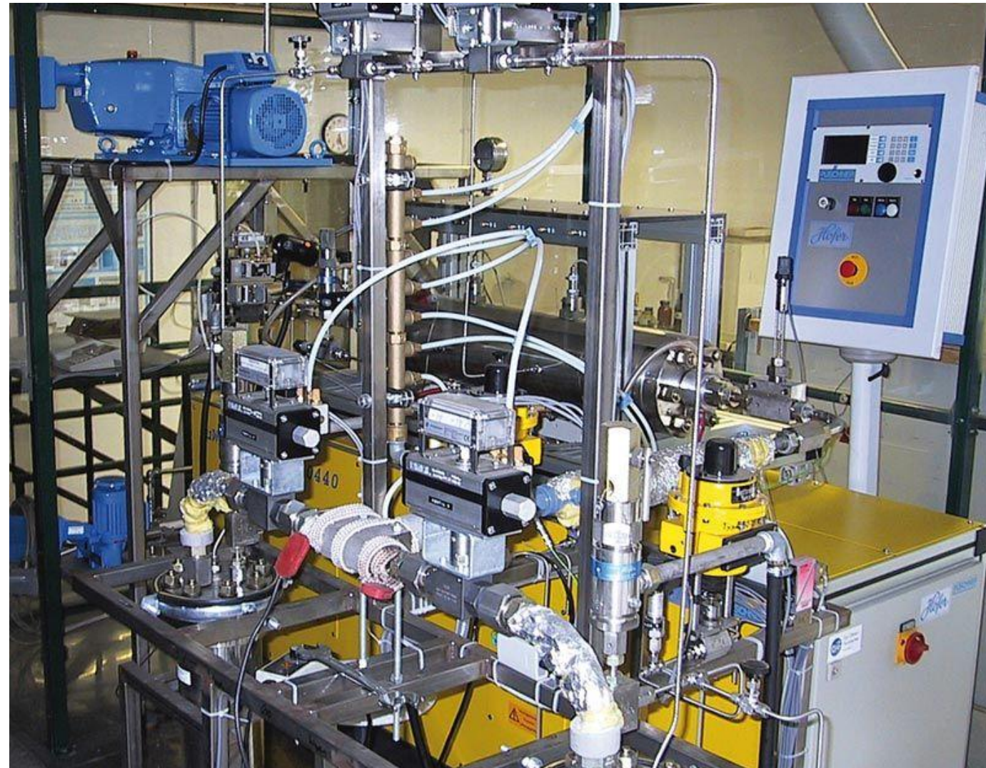
Pilot MW reactor up to 250bar/350°C
