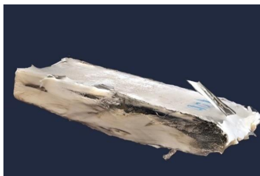
Figure 1. Cross section in a plate of 100 layers of Endumax®
