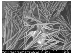
Fig. 1 – SEM micrograph of Au NWs electrochemically prepared at a cathodic potential E = -1.2 \text{ V vs. Ag/AgCl} for 1000 s at 25^\circ\text{C}
